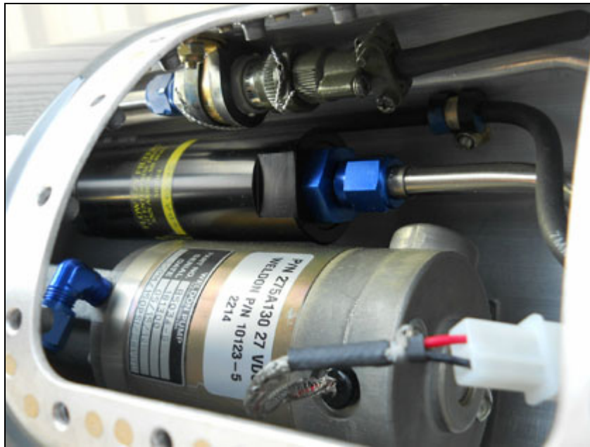
Smoke Oil Pump, Inlet Filter and Pressure Switch
